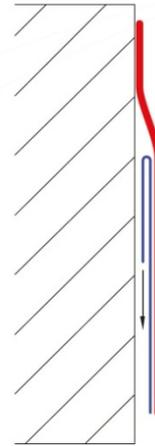
Pull release paper back at the same time pressing or rolling heater mat on to component.
