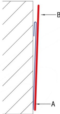
Position edge of mat against component at "A" keeping exposed adhesive away from surface at "B". When heater is in correct position, press exposed adhesive against surface at "B".
