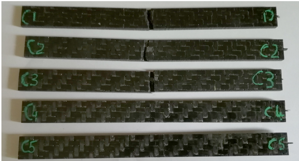
Figure 3.9 – IR specimens (top) and Convective specimens (below) following destructive testing
