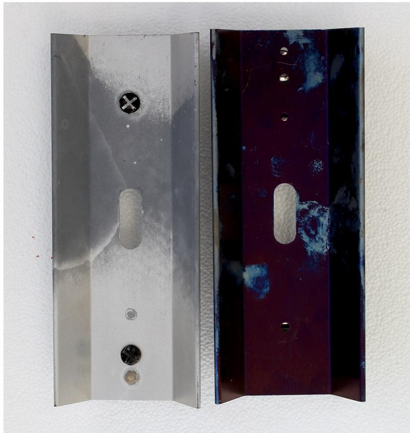
**Figure 2. Discolouration of aluminised steel (l) and stainless steel (r) reflectors caused by high-temperature exposure**
