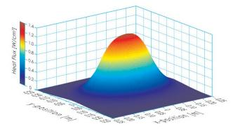
Heat flux map for FQE 1000W (Units W/cm<sup>2</sup>, 10cm from face of heater)
