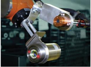
New dual head since the K Show, heat flux and non-contact IR thermocouple.
